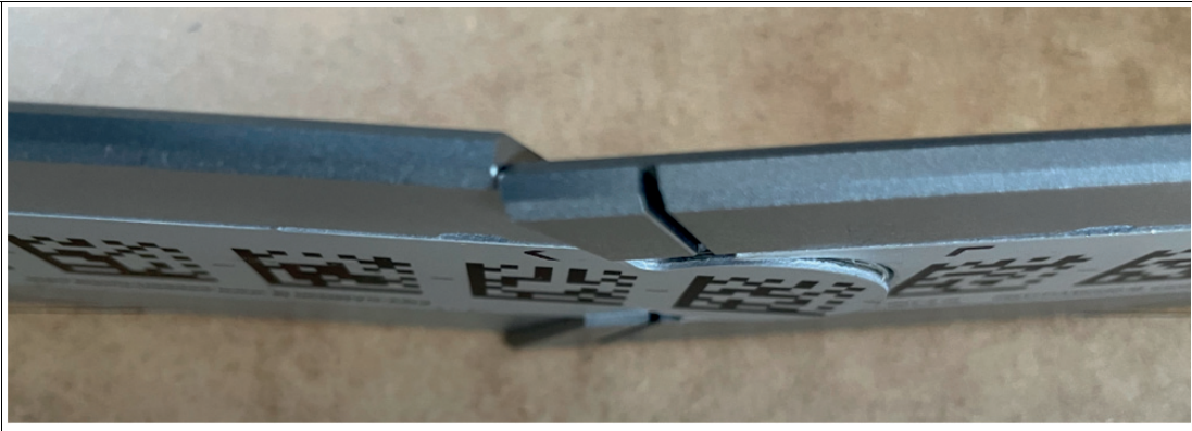
Figure 6.6 Countersunk profile rails kinked outward
