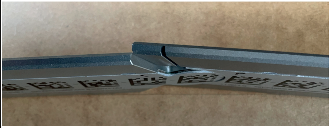
Figure 6.5 Countersunk profile rails kinked inward
